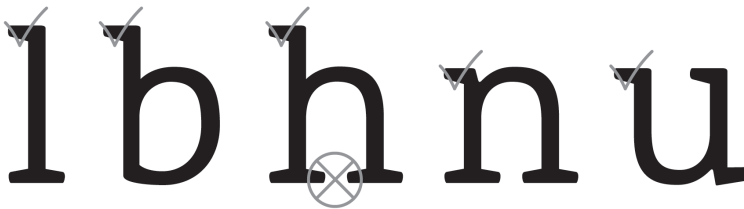
Figure 2: Beier and Dyson [2014] found that serifs on the vertical extremes improve distance legibility
