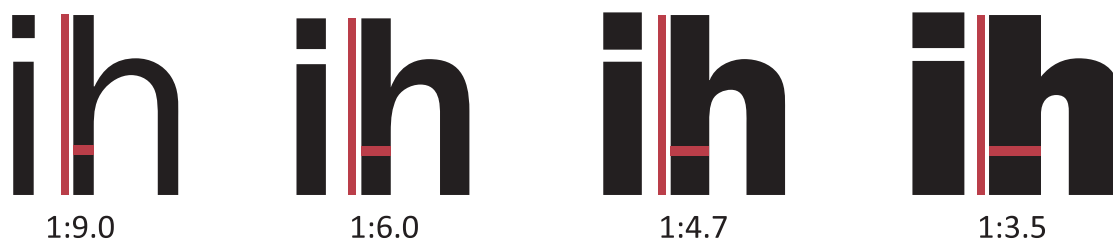
Fig. 3. Sheedy et al. (2005) tested four weights of the font family Franklin Gothic and found Franklin Gothic Book (far left) to be inferior to all the other weights in a visual acuity experiment. The stroke width/height ratio (SW/H) from left: Franklin Gothic Book (1:9.0), Gothic Medium (1:6.0), Demi (1:4.7) and Heavy (1:3.5).
