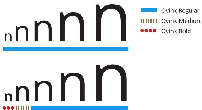
Fig. 4. Top row: all letters are set in the font weight Ovink Regular. Bottom row: The smallest letter is set in Ovink Bold, the following is set in Ovink Medium, while the three larger ones are set in Ovink Regular. In the top row, the weight appears increasingly lighter in smaller sizes, while the weight in the bottom row appears more even across the different sizes.
