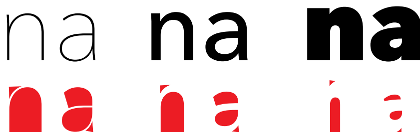
Fig. 2. The bolder the letter, the smaller the letter counter which is the area not covered by the letter stroke (marked in red). Demonstrated in the font family Avenir Next. (For interpretation of the references to colour in this figure legend, the reader is referred to the digital version of this article.)
