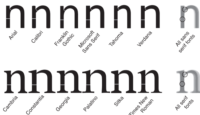
Fig. 2. A selection of the most used fonts in Windows 10. The top row shows sans-serif fonts; the bottom row shows serif fonts. By measuring the stroke contrast in the lowercase 'n' we found that the six sans-serif fonts have an average stroke contrast between thick/thin of 3/2, while the six serif fonts have an average stroke contrast of 3/0.8. Thus, the average stroke contrast in serif fonts is greater than the average stroke contrast in sans-serif fonts.
